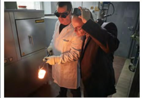
This red-hot crucible holds the molten mass of the glass-to-be, the base material for the dental prosthesis.
