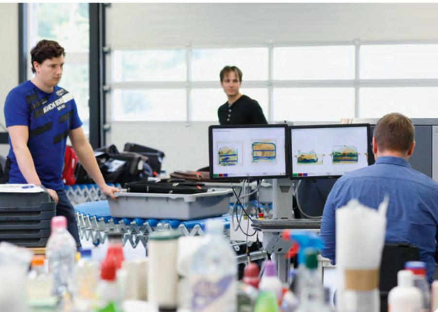
The team at Fraunhofer ICT checks whether scanner systems are able to detect hidden explosives in luggage.
