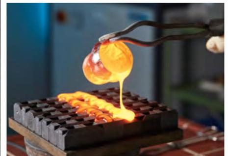
Casting and cooling the molten glass in graphite molds.
