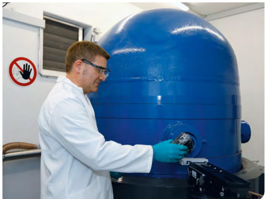
Unused explosives are disposed of in a detonation chamber weighing 20 metric tons.
