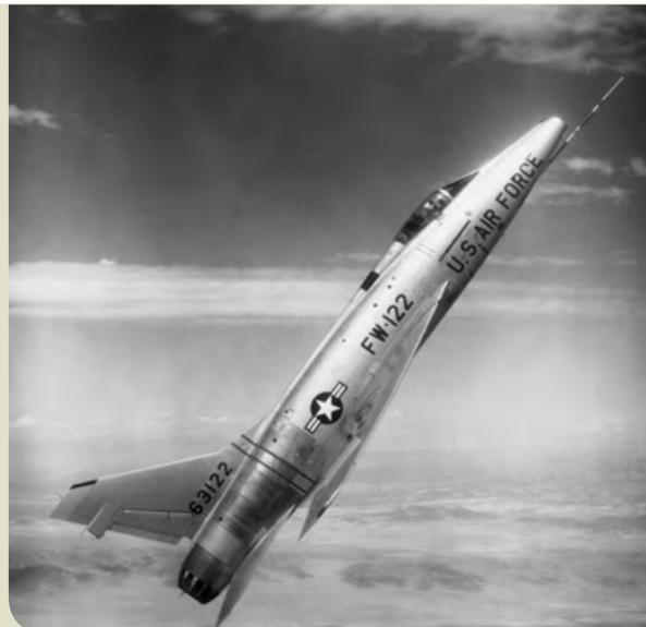
The North American F-100 belonged to the first generation of jet-engine, supersonic production aircraft and saw active service in, for example, the Vietnam War. A key advantage of the jet engine over the rocket engine is that the oxygen it requires for fuel combustion can be taken simply from the surrounding atmosphere.
