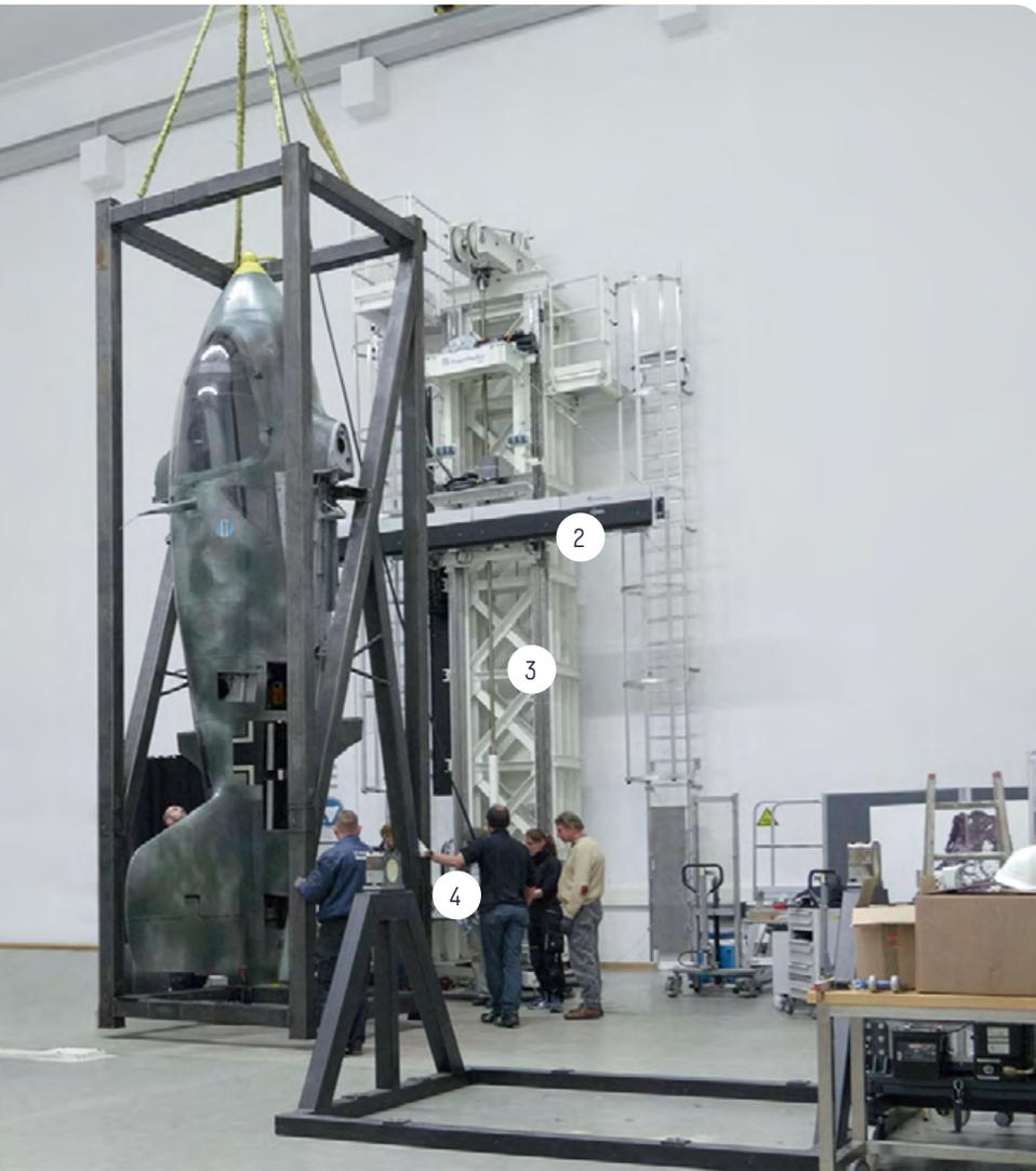
Reims and his team scanned the aircraft in an upright position, thus reducing the distance the X-rays had to penetrate. This ensured that more radiation reached the detector, thereby substantially improving the quality of the scan.
