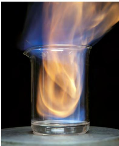
When methanol burns to form carbon dioxide and water, it gives off a blue flame with barely any soot.
