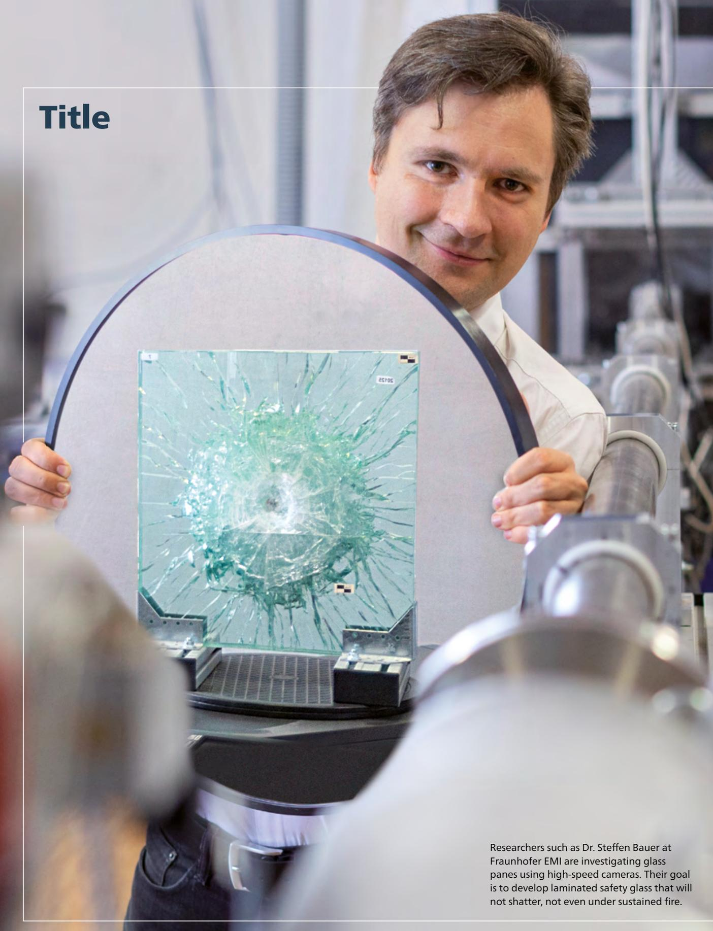
Researchers such as Dr. Steffen Bauer at Fraunhofer EMI are investigating glass panes using high-speed cameras. Their goal is to develop laminated safety glass that will not shatter, not even under sustained fire.
