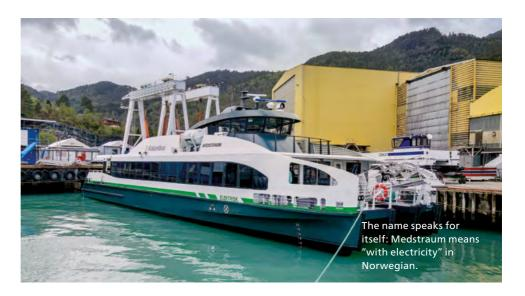
he Medstraum was developed as part of the EU project TrAM, which the Fraunhofer Institute for Mechatronic Systems Design IEM and the Fraunhofer Institute for Industrial Engineering IAO were involved in. By using modular engineering methods, the Fraunhofer researchers have been able to reduce the hours required for constructing the ferry by 70 percent, and saved 25 percent of the manufacturing costs making climate-neutral shipping cheaper.
