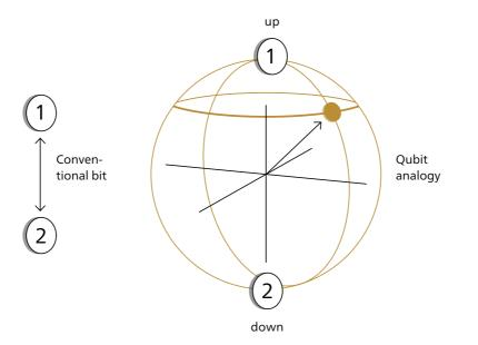
Qubits can be visualized as rotating particles, where the spin axis only settles on a fixed position when they are measured. Correlations of qubit states are used for computing.
