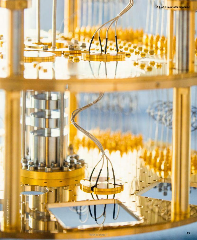
researching error correction techniques and new algorithms for practical applications, using the superconductor-based IBM Quantum System One in Ehningen.
